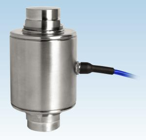
This stainless steel self-centering rocker column load cell is fully welded and hermetically sealed, with protection to IP68/IP69K. It is an ideal solution for weighbridges/truck scales thanks to its approval to OIML C4 (4000 divisions), as well as in-built lightning surge arrestors and a tough, durable polyurethane cable. Anti-rotation is achieved by means of 2 flat faces on either side of the load cell base, with corresponding flat faces in the lower mounting cup.
