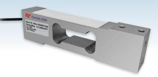
This double bending beam single point load cell is manufactured from high quality aluminium alloy. Its design allows for high accuracy weight measurement with off-centre loads. It's potted and sealed to IP66.
