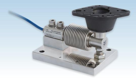
Ideal for applications with mixing, agitation and vibration, this stainless steel assembly is designed to reduce the vibration transmitted to the load cell. It is typically used in weighing platforms, big bag (FIBC) filling systems, belt weighers and hopper/tank weighing in the Food Processing, Chemical, Pharmaceutical and Bulk Handling industries.
