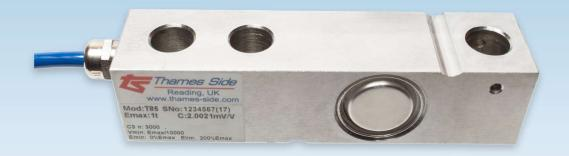
This stainless steel shear beam load cell is available with approval according to OIML R60 Class C3 (3000 divisions) and is calibrated in mV/V/ $\Omega$  by output current matching, which minimises corner correction time on multi-cell systems.
